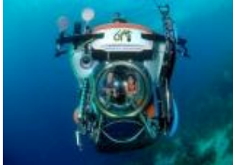
The Curasub can take its 4 passengers down to 1,000 feet
